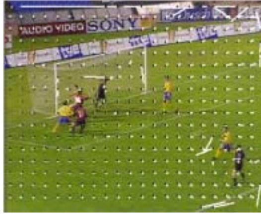
Figure 1. Block match result of two consecutive frame in a football game sequence.
