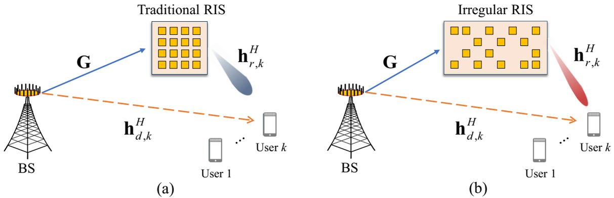
Fig. 1. The RIS-aided communication system: (a) Traditional regular RIS; (b) Proposed irregular RIS.
