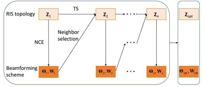
Fig. 2. The proposed joint optimization framework.
