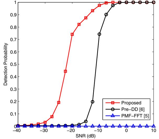
Fig. 1. Detection probability under AWGN channel with the Doppler frequency shift of 1 kHz.
