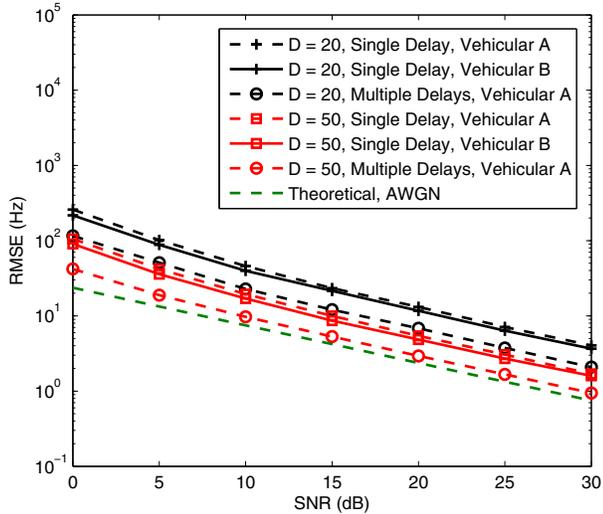
Fig. 3. Estimation accuracy of the Doppler frequency shift under multi-path channels when different delays are applied for the proposed algorithm.
