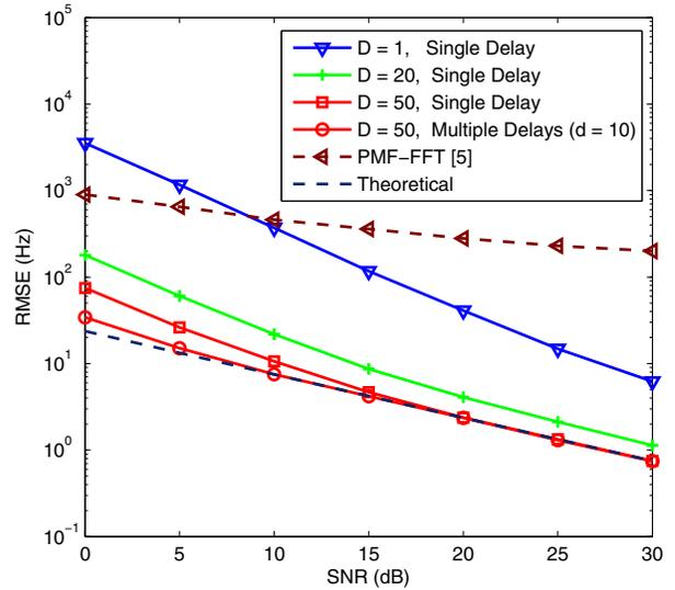
Fig. 2. Estimation accuracy of the Doppler frequency shift under AWGN channel when different delays are applied for the proposed algorithm.
