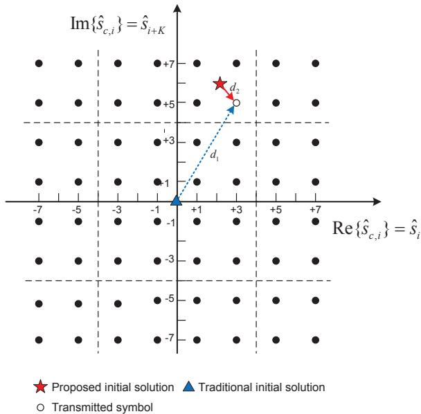
Fig. 1. Illustration of the zone-based initial solution to the Richardson method, where 64 QAM and  $Z = 4$  are considered.  $\hat{s}_{c,i}$  represents the  $i$ th element of the complex-valued estimate of transmitted signal vector  $\hat{s}_c$ .
