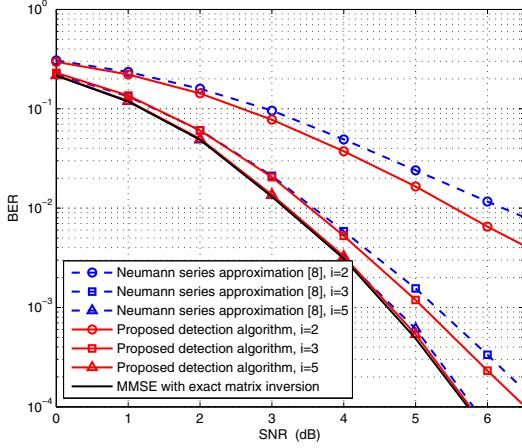
Fig. 2. BER performance comparison between the conventional Neumann series approximation algorithm and the proposed signal detection with zero-vector initial solution.
