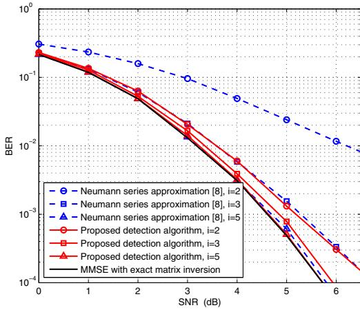
Fig. 3. BER performance comparison between the conventional Neumann series approximation algorithm and the proposed signal detection with zone-based initial solution.
