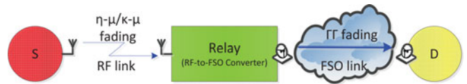
Fig. 1. The mixed RF/FSO dual-hop relay system with S, R and D denoting the source node, relay node and destination node, respectively. Moreover, the first hop (RF link) experiences a \kappa - \mu or \eta - \mu fading, and the second hop (FSO link) follows a \Gamma\Gamma fading.
