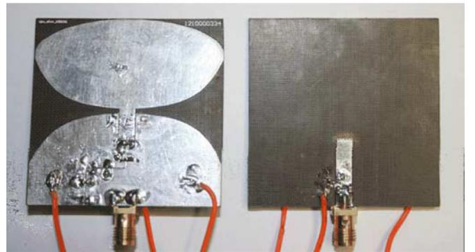
Fig. 4. Fabrication of the proposed antenna.
