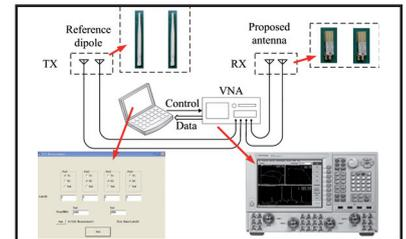
**ABOVE:** A testbench system is composed of a Vector network analyser, transmit and receive antennas, a computer and RF cables. Two reference dipoles are utilised as the transmit antennas (TX), and two test antennas are used as the receive antennas (RX). The  $2 \times 2$  antennas are connected to the 4 ports of the VNA
