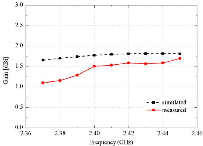
Fig. 9. Simulated and measured gain of the proposed antenna.
