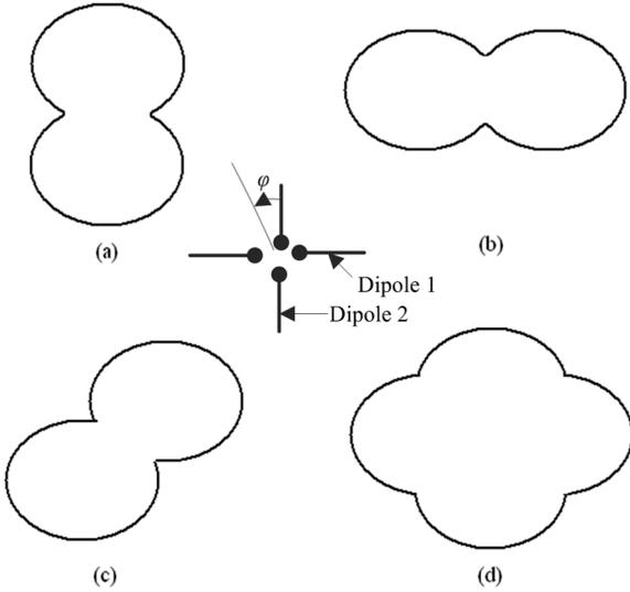
Fig. 2.  $\varphi$ -plane patterns: (a) only the dipole 1 operates; (b) only the dipole 2 operates; (c) dipoles 1 and 2 operate with the same feeding current; (d) dipoles 1 and 2 operate with the feeding current having equal magnitude and  $90^\circ$  relative phase shift.
