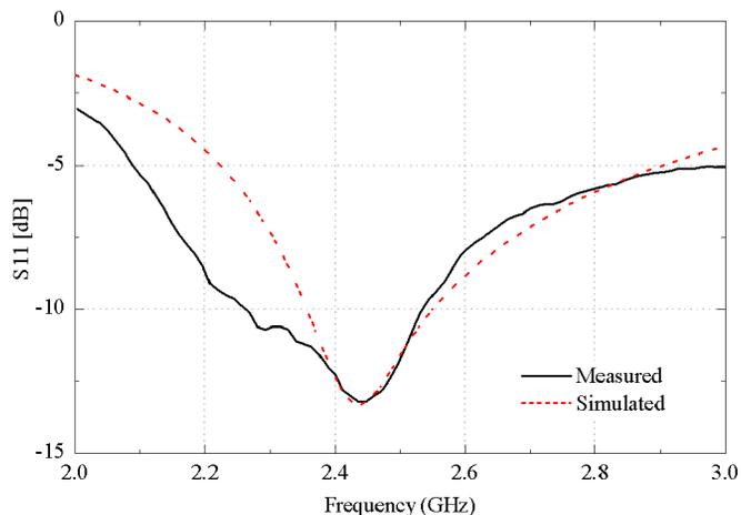
Fig. 7. Simulated and measured results of the reflection coefficient.
