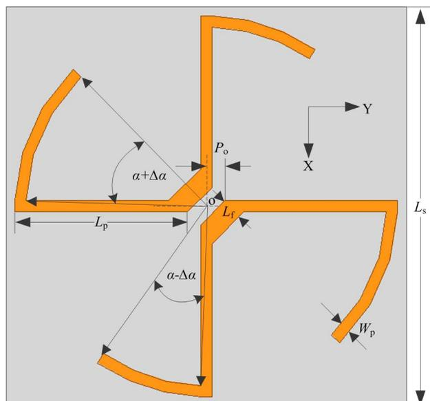
Fig. 1. Configuration of the proposed antenna.
