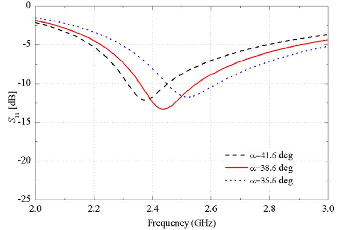
Fig. 3. Simulated reflection coefficient of the antenna for various  $\alpha$ .
