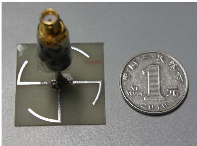
Fig. 6. Photograph of the proposed antenna.
