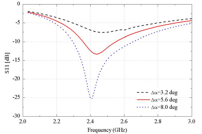
Fig. 4. Simulated reflection coefficient of the antenna for various  $\Delta\alpha$ .
