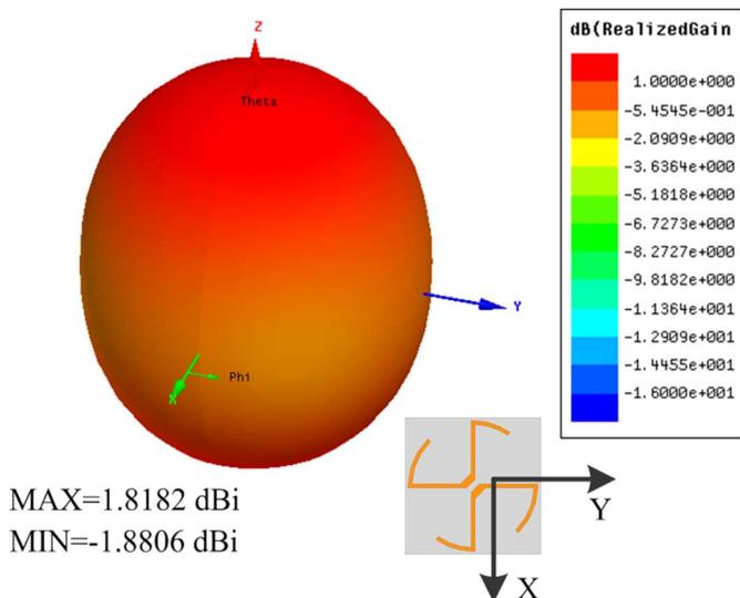
Fig. 5. Three-dimensional simulation radiations pattern of the antenna at 2.44 GHz.
