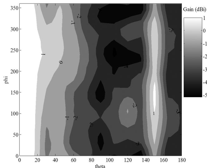
Fig. 8. Gain contour lines at 2.4 GHz.
