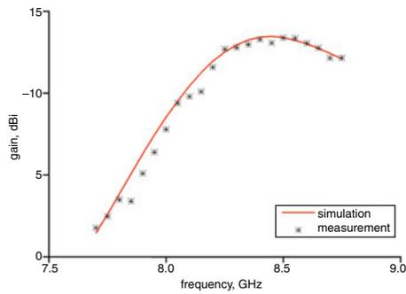
**Fig. 5** Measured and simulated gains at broadside
