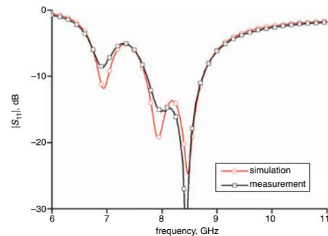
Fig. 4 Measured and simulated magnitude of reflection coefficients
