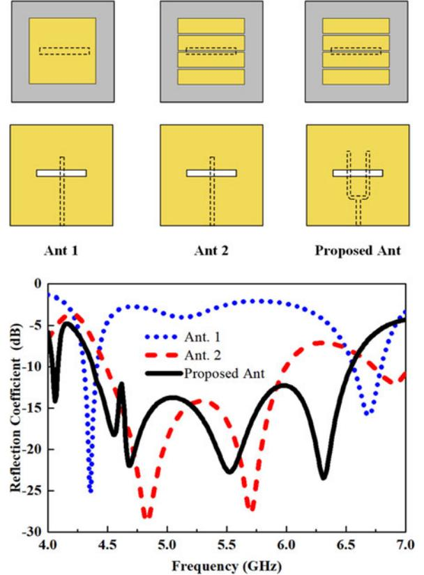
Fig. 2. Geometries and simulated reflection coefficients of the three antennas with different radiating patches and feeding structures.
