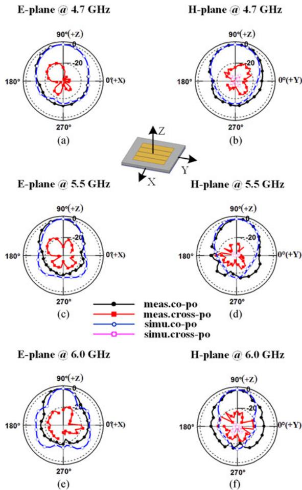
Fig. 7. Simulated and measured normalized radiating patterns of the proposed microstrip antenna at 4.7, 5.5 and 6 GHz in *E*-plane and *H*-plane.
