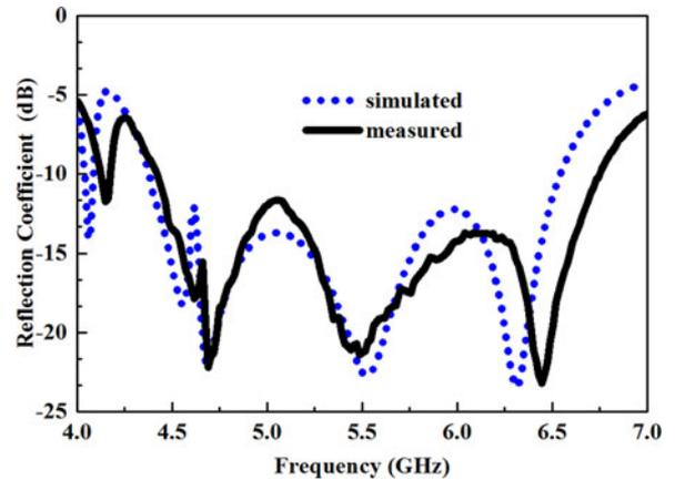
Fig. 5. Simulated and measured reflection coefficients of the proposed microstrip antenna.
