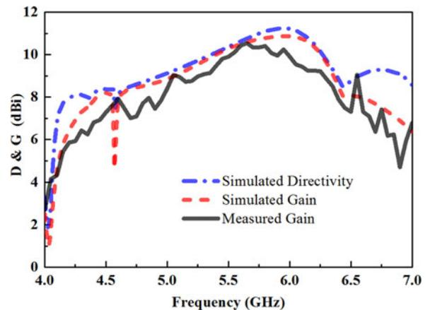
Fig. 6. Simulated directivity, simulated gain and measured gain of the proposed microstrip antenna.
