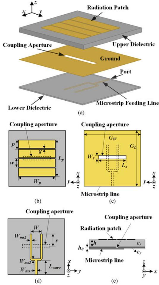
Fig. 1. Geometry and dimensions of the proposed antenna: (a) Perspective view of the layered structure, (b) top layer of the radiating patch with strip-slot hybrid structure, (c) middle layer of the ground with the coupling aperture, (d) bottom layer of the Y-shaped feeding microstrip line. (e) Side view of the overall structure.
