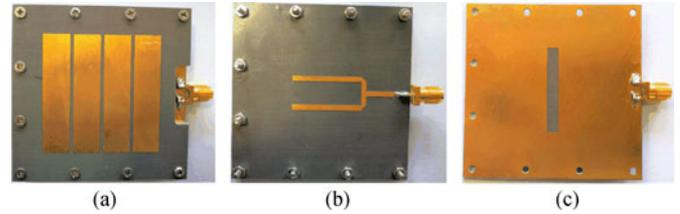
Fig. 4. Photographs of the fabricated antenna: (a) top layer of the radiating patch with strip-slot hybrid structure, (b) Y-shaped microstrip feeding line in the bottom layer, and (c) middle layer of the ground with the coupling aperture.
