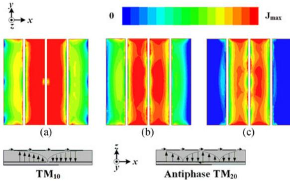
Fig. 3. Current distributions and operating modes of the proposed antenna at different resonances: (a) 4.7 GHz. (b) 5.5 GHz. (c) 6.3 GHz.
