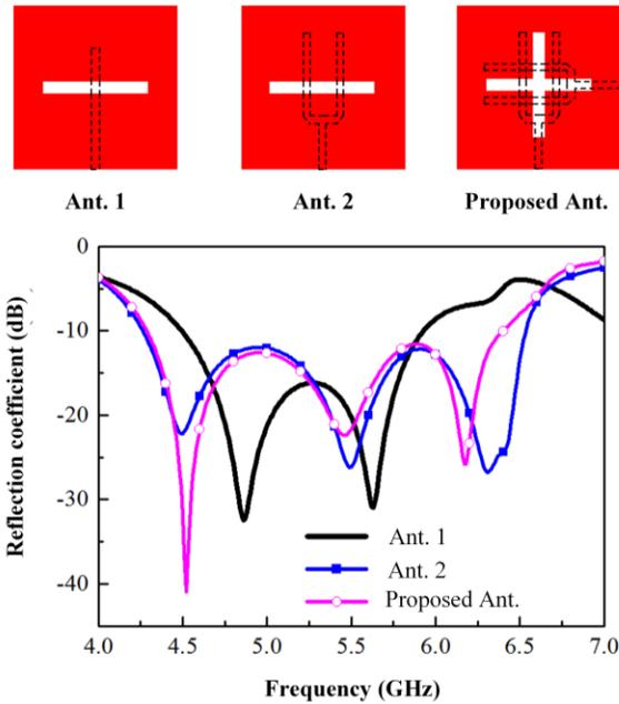
Fig. 3. Design evolution and simulated reflection coefficients.
