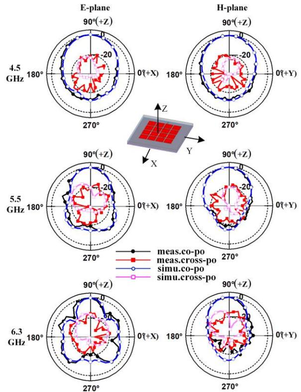
Fig. 7. Simulated and measured normalized radiating patterns at port 1 of the Proposed Ant. at 4.5 GHz, 5.5 GHz and 6.3 GHz.
