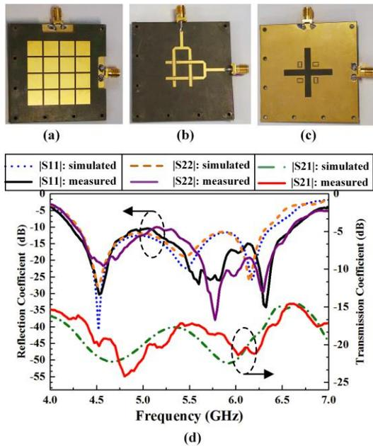
Fig. 6. Photographs and measured results of the fabricated Proposed Ant. (a) Top view, (b) bottom view, (c) the ground plane and cross coupling apertures in the GND layer, and (d) simulated and measured reflection and transmission coefficients.
