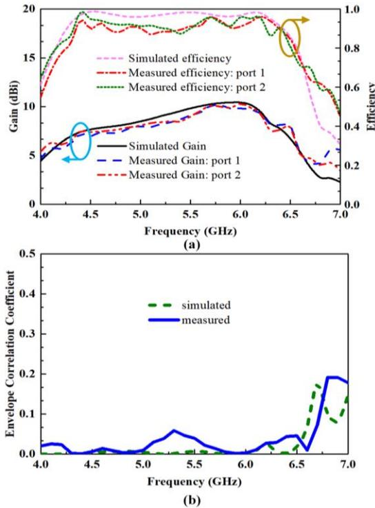
Fig. 9. Simulated and measured radiating performances of the Proposed Antenna. (a) Gain and efficiency, and (b) envelop correlation coefficients.
