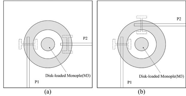
Fig. 2. Two different feeding configurations for P1 and P2: (a) T-shaped arrangement of slots; (b) L-shaped arrangement of slots.
