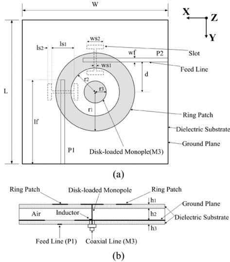
Fig. 1. Geometry of the tripolarization antenna: (a) top view; (b) side view.
