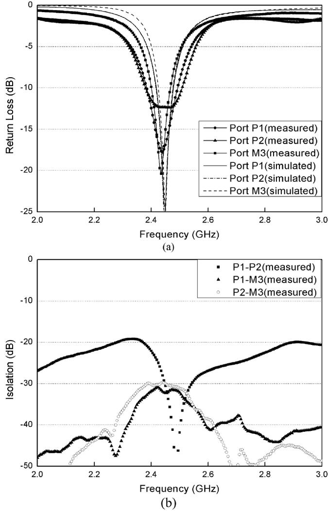
Fig. 4. Measured and simulated  $S$ -parameters of the tripolarization antenna ports: (a) return loss; (b) isolation.
