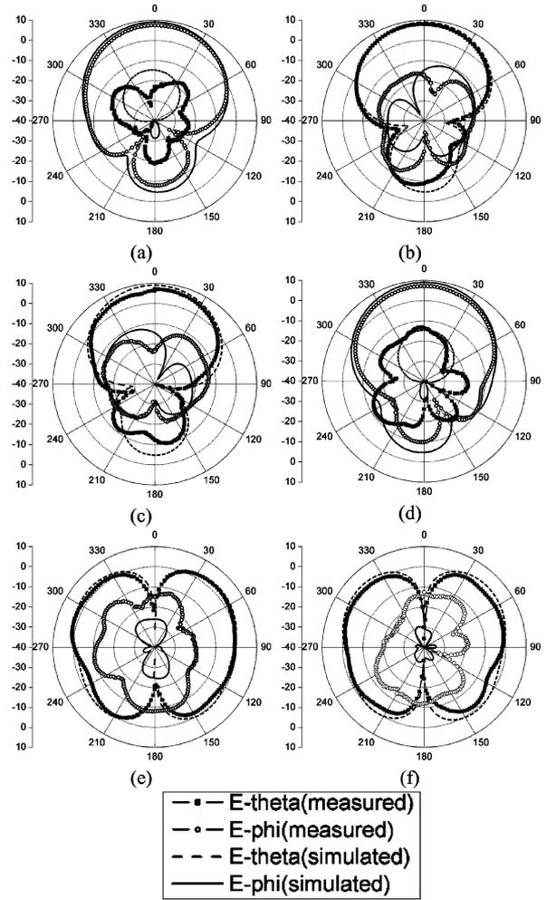
Fig. 5. Measured and simulated gain patterns of the tripolarization antenna. (a) Port P1,  $xz$  plane. (b) Port P1,  $yz$  plane. (c) Port P2,  $xz$  plane. (d) Port P2,  $yz$  plane. (e) Port M3,  $xz$  plane. (f) Port M3,  $yz$  plane.
