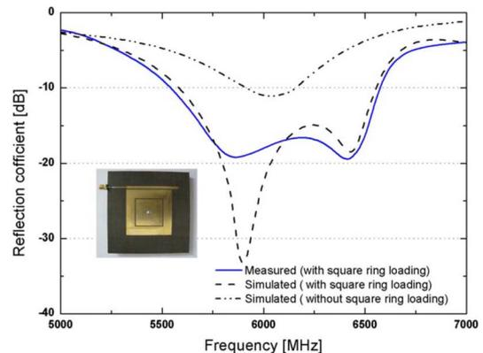
Fig. 7. Measured and simulated reflection coefficient  $S_{22}$  for ITS operation.
