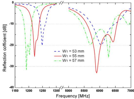
Fig. 3. Simulated reflection coefficient for different width  $W_1$  of the outer square ring.
