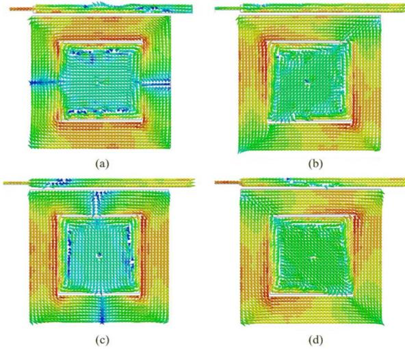
Fig. 2. Snapshots of the simulated current distribution of the proposed antenna at different phase values. (a)  $\Delta\varphi = 0^\circ$ . (b)  $\Delta\varphi = 45^\circ$ . (c)  $\Delta\varphi = 90^\circ$ . (d)  $\Delta\varphi = 135^\circ$ .
