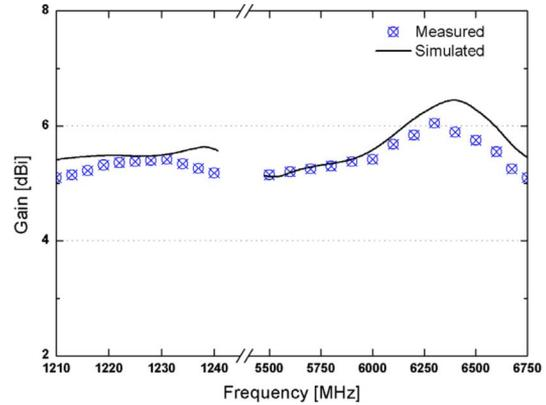
Fig. 11. Measured and simulated antenna gain of the multifunctional antennas.
