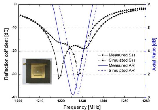
Fig. 6. Measured and simulated reflection coefficient  $S_{11}$  and axial ratio for GSP operation.
