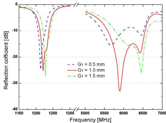
Fig. 4. Simulated reflection coefficient for different width  $G_1$  of the narrow slot.
