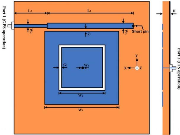
Fig. 1. Geometry of the proposed GPS/ITS integrated antenna.
