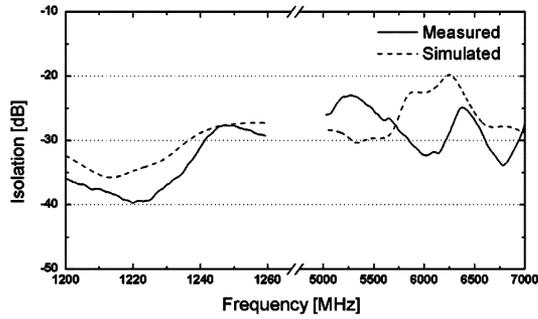
Fig. 8. Measured and simulated isolation between the feeding ports of GPS operation and ITS operation.
