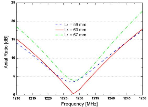
Fig. 5. Simulated axial ratio for different length  $L_1$  of the short-ended microstrip line.
