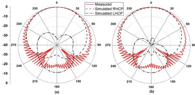
Fig. 9. Measured and simulated radiation patterns of the integrated GPS antenna at 1227 MHz. (a)  $xz$  plane. (b)  $yz$  plane.
