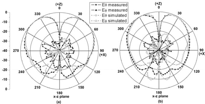
Fig. 10. Measured and simulated radiation patterns of the integrated ITS antenna. (a) 5.7 GHz. (b) 6.4 GHz.
