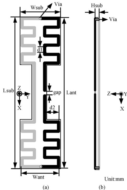
Fig. 4. Geometry of the proposed element. (a) Top view. (b) Side view (the dark line is printed on the top layer, while the gray is printed on the bottom layer).
