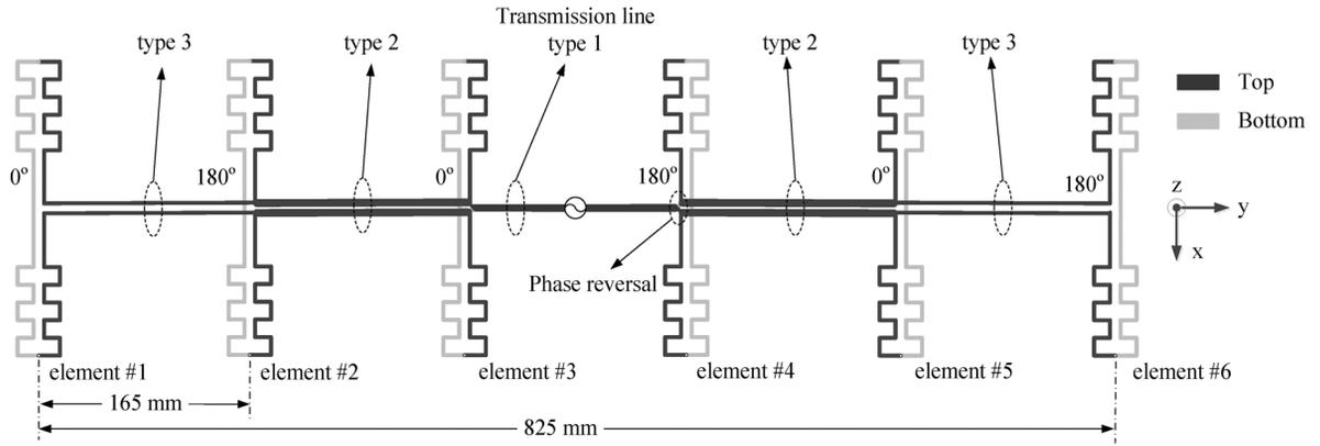
Fig. 1. Schematic of the proposed array.
