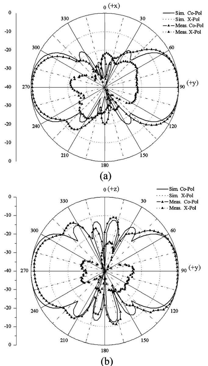
Fig. 7. Simulated and measured normalized radiation patterns at 860 MHz for the proposed array. (a)  $xy$ -plane. (b)  $yz$ -plane.
