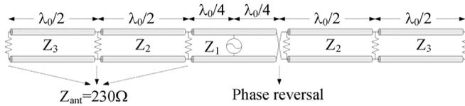
Fig. 2. Equivalent circuit model of the proposed array.
