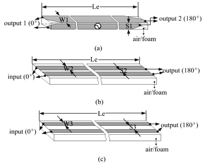
Fig. 3. Schematic of the transmission line structure. (a) Type 1. (b) Type 2. (c) Type 3 (unit: millimeters, not in scale).
