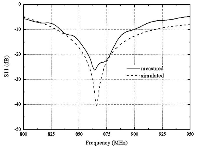
Fig. 6. Simulated and measured  $S_{11}$  for the proposed array.
