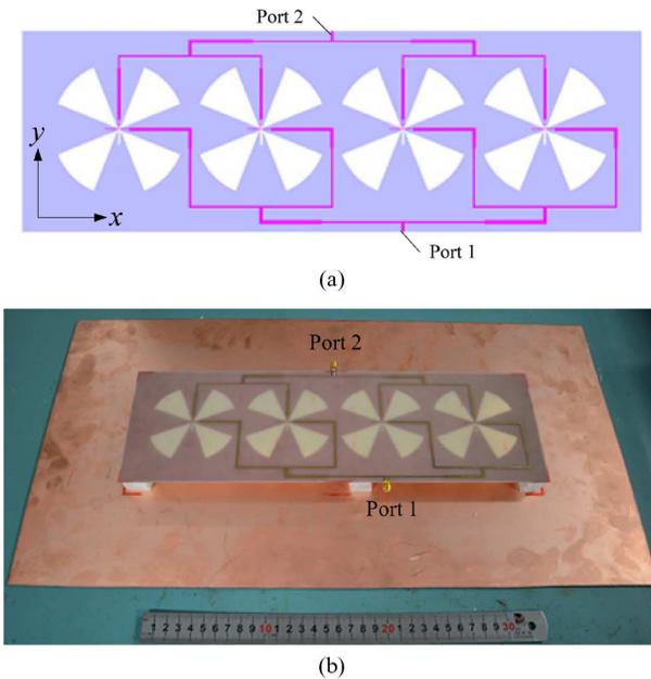
Fig. 5. Dual-polarized array antenna: (a) Top view. (b) Prototype.
