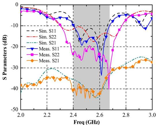
Fig. 6. Measured and simulated  $S$ -parameters of the proposed array antenna.
