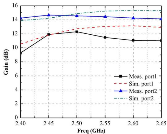
Fig. 10. Measured and simulated gain of the proposed array antenna.
