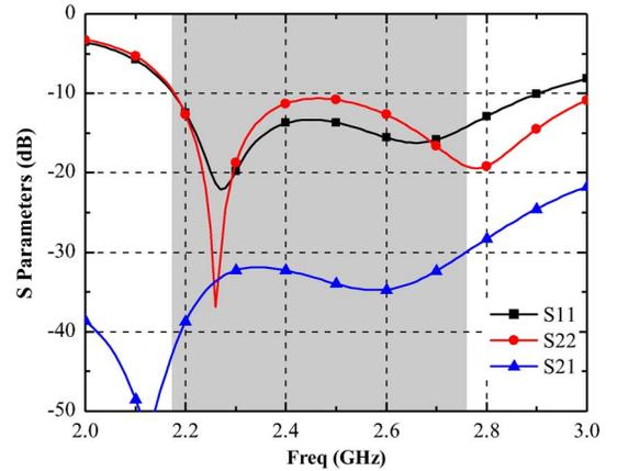
Fig. 4. Simulated  $S$ -parameters of the proposed element antenna (normalized impedance value equals  $120 \Omega$ ).
