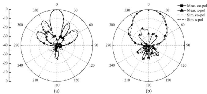
Fig. 9. Measured and simulated radiation patterns of Port 2 feeding at 2.5 GHz: (a)  $xz$ -plane; (b)  $yz$ -plane.
