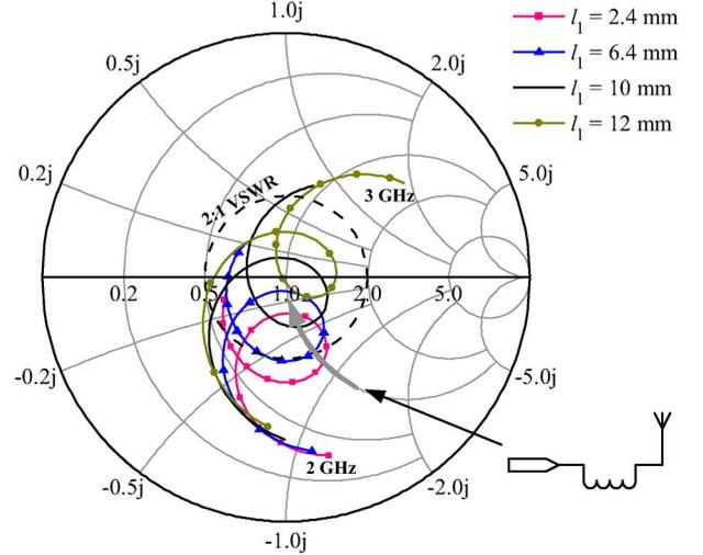
Fig. 3. Impedance curves of  $0^\circ$  polarized element antenna on Smith chart with different  $l_1$  (fed at point A as shown in Fig. 1, normalized impedance value equals  $120 \Omega$ ).
