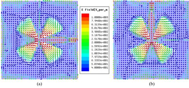
Fig. 2. Electric field distribution of element antenna at 2.5 GHz: fed from (a) Port 1 and (b) Port 2.
