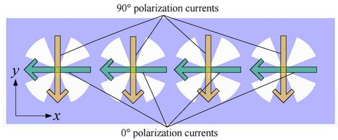
Fig. 7. Current direction of the two polarizations on each element.
