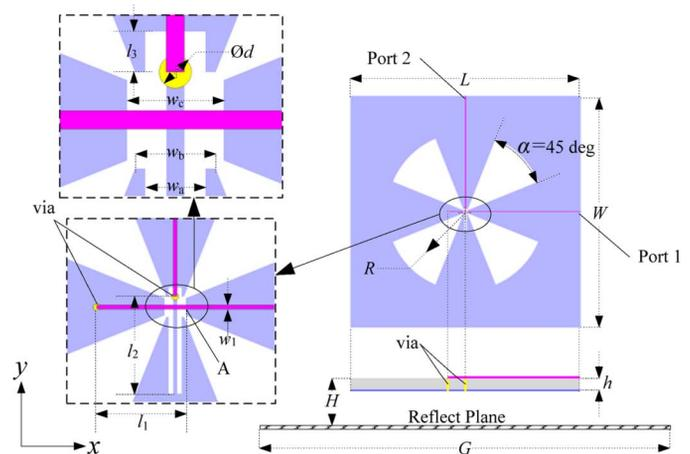
Fig. 1. Geometry and description of the proposed element antenna.
