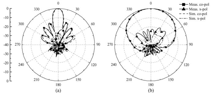
Fig. 8. Measured and simulated radiation patterns of Port 1 feeding at 2.5 GHz: (a)  $xz$ -plane; (b)  $yz$ -plane.
