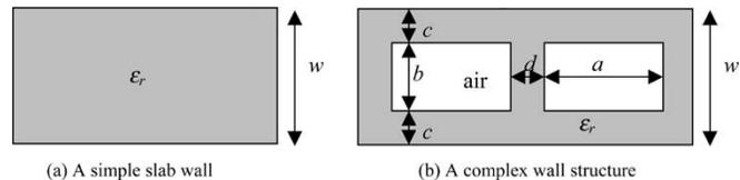
Fig. 1. Simple slab walls and complex walls used in the simulation. (a) Simple slab wall. (b) Complex wall structure.
