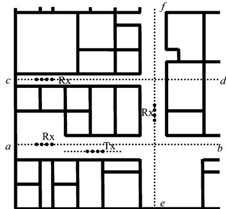
Fig. 6. Linear antenna array geometry for the MIMO capacity calculations. Tx and Rx are the transmit and receive MIMO arrays. (a) Normalized capacity for complex walls. (b) Normalized capacity for slab walls. (c) Normalized capacity for effective walls.
