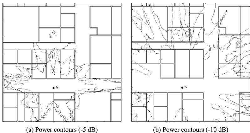
Fig. 3. Comparisons of equal-power patterns between (solid line) the complex, (dashed line) slab walls, and (dotted line) effective walls. (a) For  $-5$ -dB power contours. (b) For  $-10$ -dB power contours.
