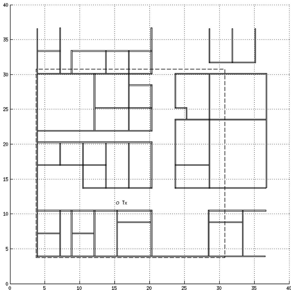
Fig. 2. FDTD model for a floor plan in a building. The whole FDTD model has a dimension around  $40 \times 40$  m. The fields in the dashed rectangle (around  $27 \times 27$  m) will be analyzed. All dimensions are in meters.
