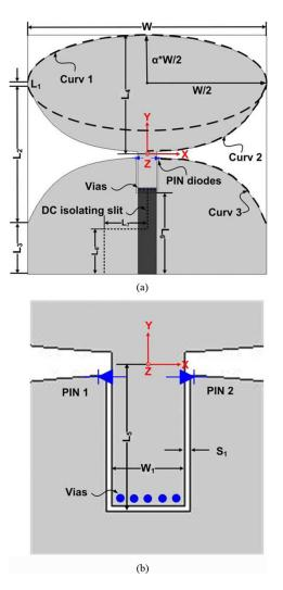
Fig. 1. Geometry and configuration of the proposed antenna. (a) Front view. (b) Detailed view of feed structure.
