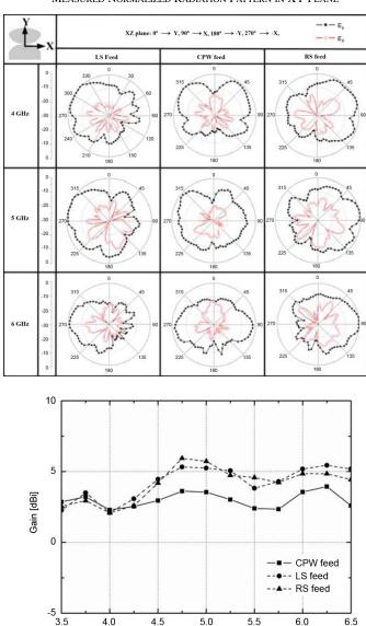
Fig. 8. Measured gains of antenna through different feed.
