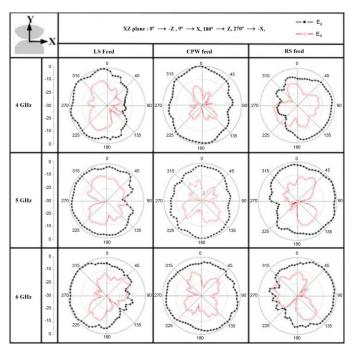
a nearly omni-directional radiation pattern is achieved in XZ plane and a doughnut shape in XY plane. For the LS or RS feed, a unidirectional beam is achieved along -X or +X axis, with acceptable front-to-back ratio better than 9.5 dB. The different patterns of radiation are able to be switched dynamically according to the environment, proving the pattern diversity.
