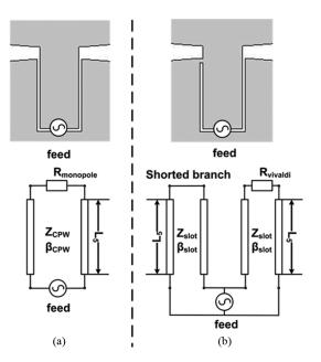
Fig. 2. Feed diagram and equivalent transmission line model. (a) CPW feed (b) RS feed.
