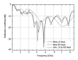
Fig. 7. Simulated and measured reflection coefficients of slotline feed.
