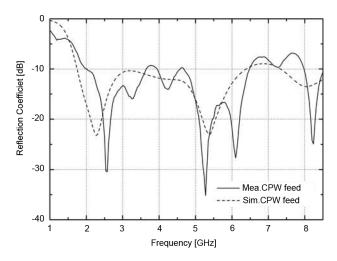
Fig. 6. Simulated and measured reflection coefficients of CPW feed.
