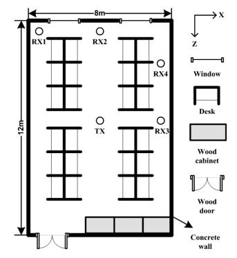
Fig. 9. Indoor environment for channel capacity measurement.
