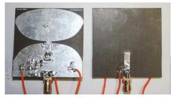
Fig. 4. Fabrication of the proposed antenna.
