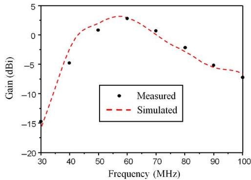
Fig. 16. Measured and simulated gain results of the dynamic-type shunt-excited sea-water monopole antenna.
