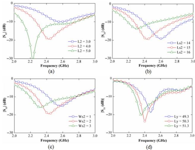
Fig. 3. Magnitude of reflection coefficients with variation of (a)  $L_2$ , (b)  $L_{s2}$ , (c)  $W_{s2}$  for the dipole mode, and (d)  $L_y$  for the patch mode (unit: millimeter).
