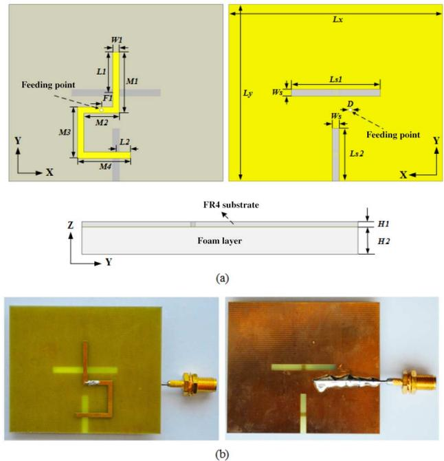
Fig. 1. Geometry of the proposed antenna and the prototype.
