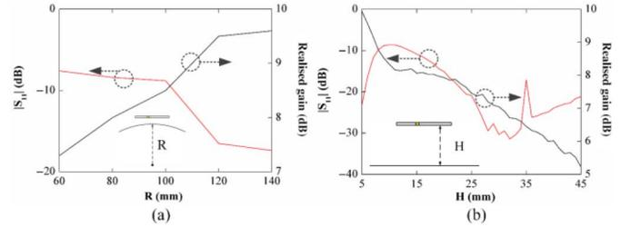
Fig. 4. Magnitude of reflection coefficients and realized gains at broadside at 2.4 GHz with variation of (a)  $R$  and (b)  $H$ .
