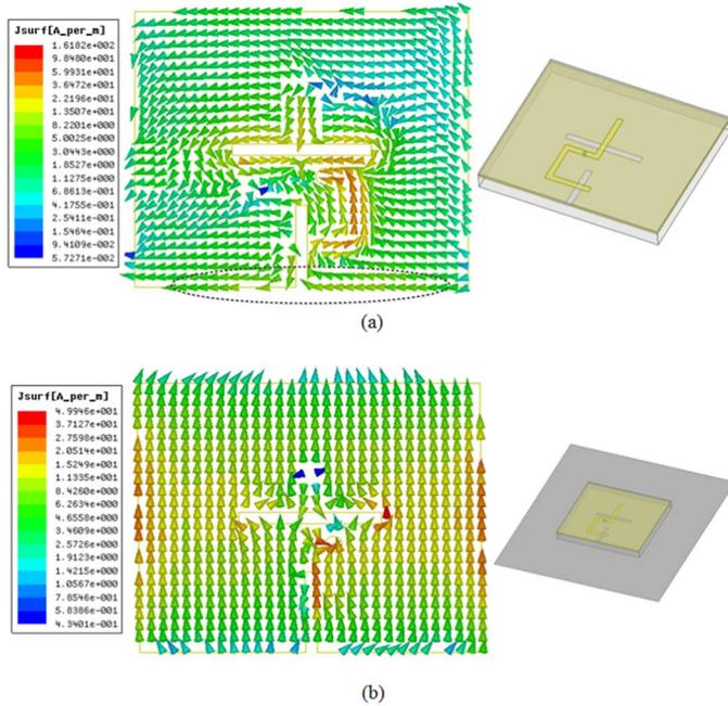
Fig. 2. Current distributions of the two operating modes at 2.4 GHz. (a) Dipole mode in free space. (b) Patch mode on a metallic surface.
