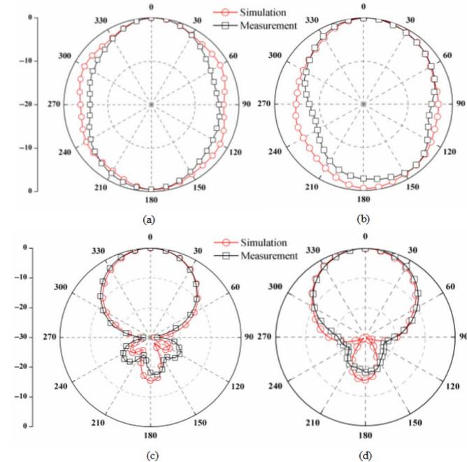
Fig. 6. Measured and simulated radiation patterns of the proposed antenna at 2.4 GHz: the dipole mode in (a) E-plane and (b) H-plane, and the patch mode in (c) E-plane and (d) H-plane.
