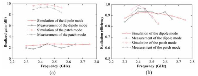
Fig. 7. Measured and simulated (a) peak gains and (b) radiation efficiencies of the proposed antenna.
