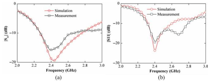
Fig. 5. Measured and simulated magnitude of reflection coefficients of the proposed antenna. (a) Dipole mode. (b) Patch mode.
