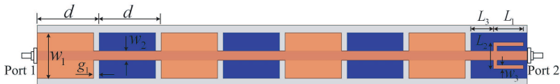
Figure 9. Geometry of the proposed 5.8 GHz antenna array with a fork shape stub.
