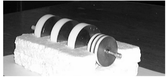
Fig. 2. Photograph of fabricated multiband six-element coaxial CTS antenna array designed to operate at 4.2 and 19.4 GHz: angled view.
