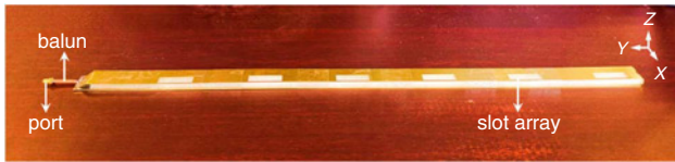
Fig. 5 Photograph of proposed slot array
